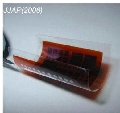
Flexible aSi solar cell (on PET), Efficiency ~6%
